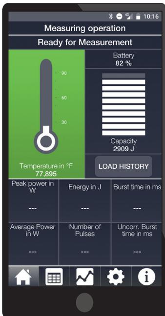
Using the PRIMES Cube App for mobile devices with Android™, you can operate and monitor all Cube models simply and conveniently on a tablet or smartphone via Bluetooth. Entire measuring series can be preset through the user-friendly interface on the mobile terminal and transmitted wirelessly to the Cube. It will graphically display the measuring values of laser power, pulse duration, and collected energy per pulse on the mobile terminal.
