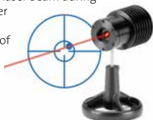
LM-45 HTD sensor with beam position
