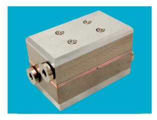
A Taranis module can amplify a pulsed seed laser from a few kHz to several tens of MHz, or a seed laser from ten's of nanoseconds down to a few hundred of femtoseconds with seed powers ranging from a few hundred of mWatts up to tens of Watts.
