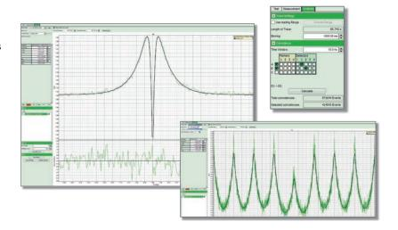
The QuCoa software package is an integrated solution for data acquisition and analysis using PicoQuant's TCSPC electronics in their unique T2 time-tagging mode. It is mainly targeted at all research areas that rely on coincidence detection such as Hanbury-Brown-Twiss setups to study single photon sources ( $g^{(2)}$  / antibunching), quantum key distribution (QKD), or the study of entanglement using Hong-Ou Mandel (HOM) setups, to name only a few.
